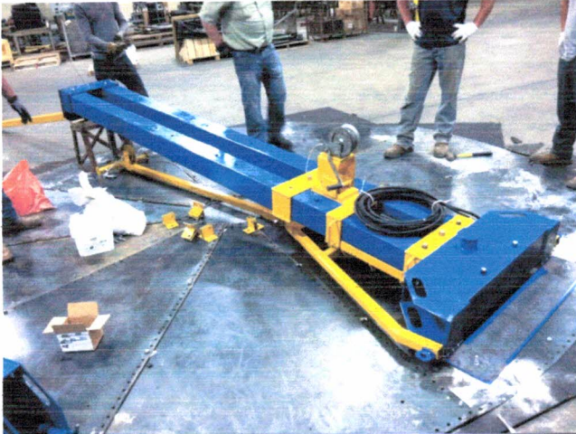
Elevate head of jack to allow yoke placement
