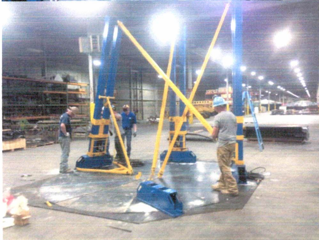
Raise jack with winch, attach strut.
