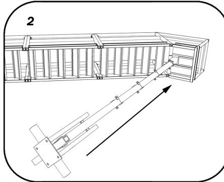
Slide the 4"x4"x5' pole piece over the base. (see fig 1) Note that the 4 round washers go toward the top. Slide in additional 4"x4" pieces as
