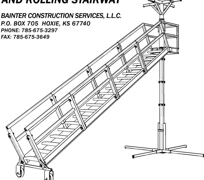
Thank you for your purchase of the Bainter Center Ring Support and Rolling Stairway. We are here to serve your grain bin construction needs with equipment that makes your work easier, faster, and safer.
