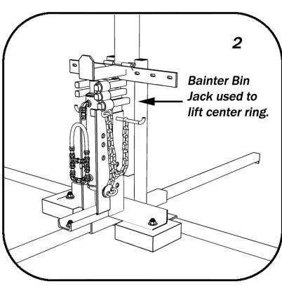
After The center ring is in place, raise the center pole to the correct height. This can be accomplished in two ways. A cable winch can be used as pictured above (fig 1), or a "Bainter" hydraulic bin jack in the 32" position can be used by placing the bolt strap under the bracket welded to the side of the 5' starter pole. as pictured at left (fig 2).
