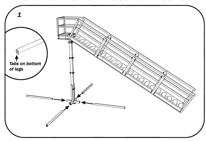
Immediately slide the legs into the receivers on the base. The steel tabs on the ends of the legs must face downward to prevent teetering of the tower.
