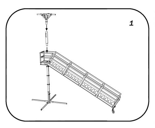
After the stairway is raised and the extension legs are slipped in place, the Center Ring support pieces should be installed at the landing
