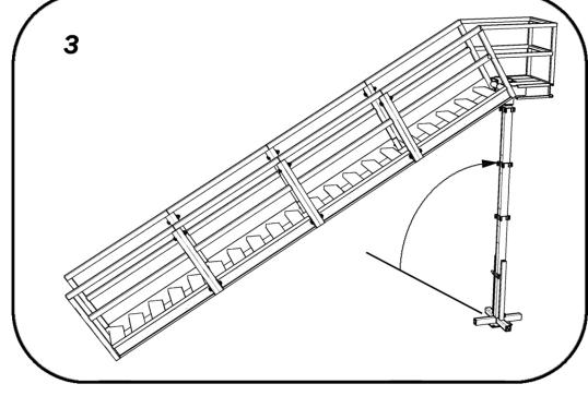
Raise the tower and stairway to it's vertical position. (see fig. 3) This can be done without additional lifting equipment on systems for 60' Dia. and smaller.
